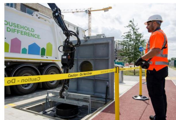
Innovative underground waste and recycling system conceals refuse bins, reducing visual impact and odour, damage from weather, and helps to avoid attracting pests.
